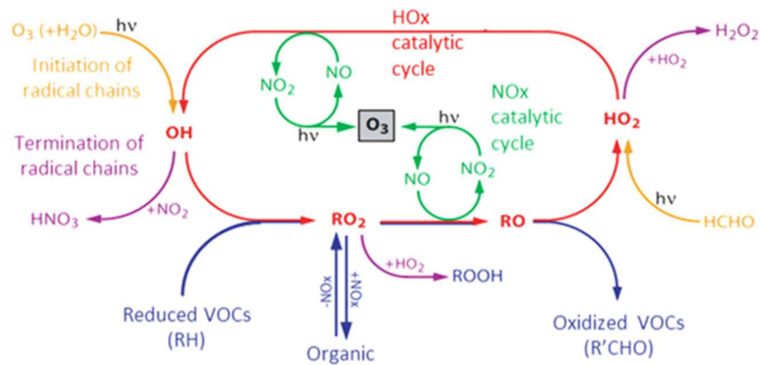
Figure 2.35 – Schematic representation of the main mechanisms involving nitrogen dioxides in the troposphere (Aumont, 2015).
