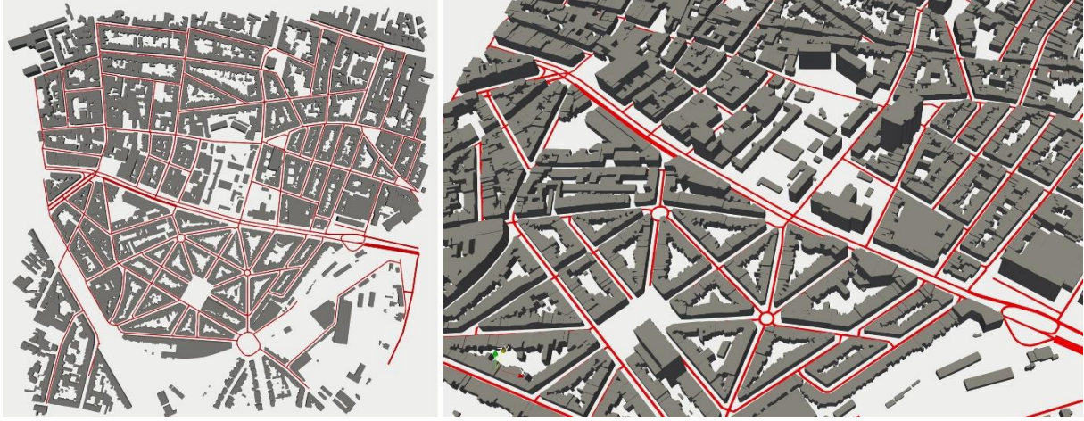
Figure 3. Overview of the 3D numerical model with (A) a top view and (B) a three-quarter view (red lines correspond to roads for which emission data were available and were modeled).
